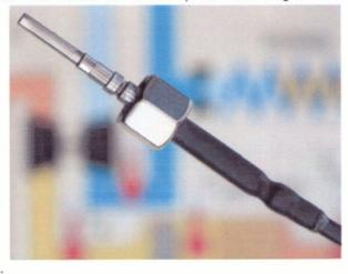
Based on a proven mineral insulated thermometer, the *M-TS* will be assembled with flexible production methods in a support sleeve and then be sealed. Those methods enable EngineSens to customize smaller requirements to individual needs and still match demanding cost targets. It is fixed by means of male or female nuts. This eliminates the hassle of turning the sensor during installation. Cable lengths, immersion depths, connector and mounting options are customized.
